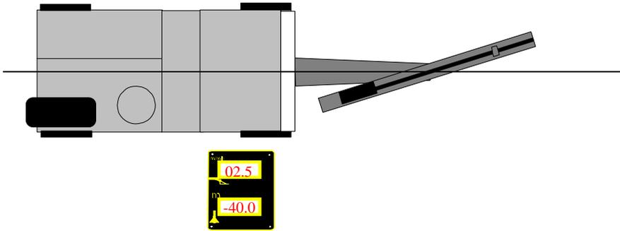
In **relative mode** both angles are related to the preset angles. This function makes it very easy to drill parallel holes:
